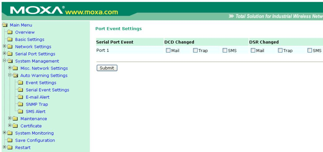
On the Serial Event Settings page, you may configure how administrators are notified of each serial port’s DCD and DSR changes. Mail refers to sending an e-mail to a specified address. Trap refers to sending an SNMP Trap. DOUT refers to changing the status of the relay output. SMS refers to sending a message to one or more specified phone numbers.
